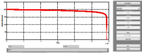
Fig. 2 Radial distance of the satellite with increasing time
